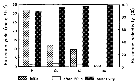
FIG. 11. Performance of catalysts of the series \text{XPV}_2\text{Mo}_{10}\text{-Pd} , where X = \text{H}^+ , \text{Cu}^{2+} , \text{Ni}^{2+} , and \text{Cs}^+ , in the oxidation of 1-butene at 343 K.
